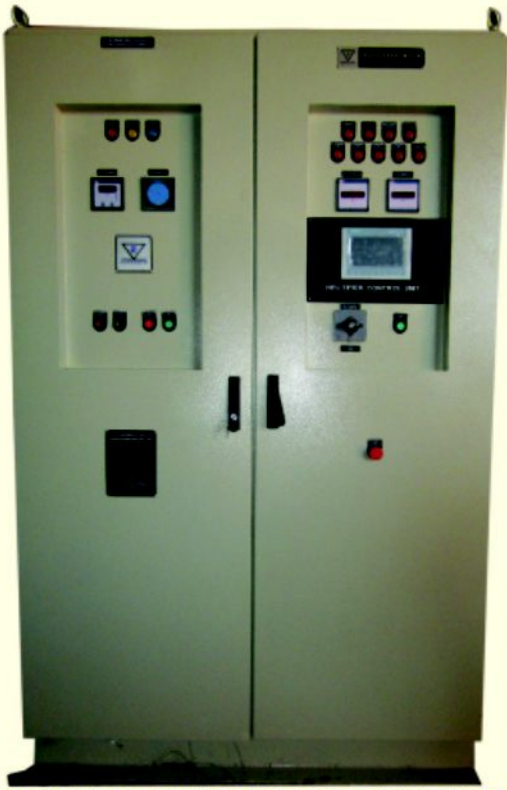
SUPPLY OF 12V / 10KA SCR CONTROLLED (12 PULSE) RECTIFIER TO HINDALCO FOR ELECTRO MAGNETIZING PROCESS IN ALUMINIUM SMELTER
