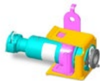
Variable expansion dampers ( VED) significantly improving the NVH parameters
