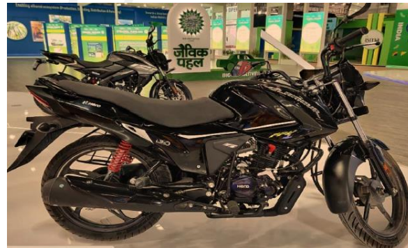
The Hero Glamour Xtec has a 125cc engine, 10L fuel tank and compatibility of E20-E85 ethanol mix
