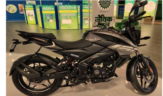
Bajaj Pulsar Ns160 flex fuel has 12L fuel tank capacity and can work in the E20-E85 range
