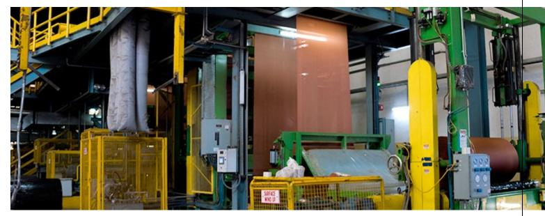
Greige fabric has very poor adhesion to rubber. Therefore, it is impregnated with an RFL (Resorcinol - Formaldehyde - Latex) solution which acts as a bonding agent between fabric and rubber.
