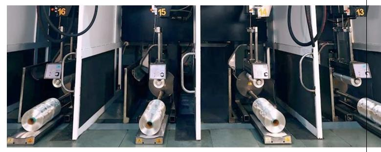
Here Dried chips are fed into a melt spinning machines. The molten polymer is filtered before entering the spinneret (a wheel or plate with many tiny holes) to form yarn of different linear density as per specifications.
