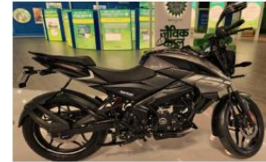
Bajaj Pulsar Ns160 flex fuel has 12L fuel tank capacity and can work in the E20-E85 range
