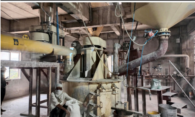
Fig 3 – Raw material mixer where fly ash, water, cement and lime are mixed to form AAC slurry
